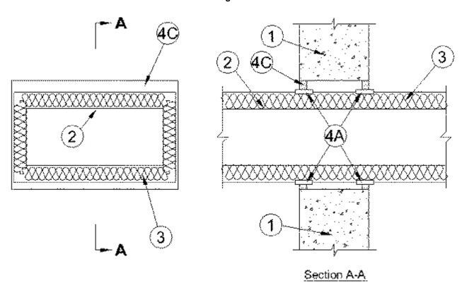
1. **Wall Assembly** — Min 6-1/8 in. (156 mm) thick reinforced lightweight or normal weight (100-150 pcf or 1600 - 2400 kg/m³) concrete wall. Wall may also be constructed of any UL Classified **Concrete Blocks**\*. Max area of opening is 900 sq in. with max dimensions of 30 in.
