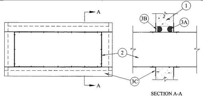
1. **Wall Assembly** — Min 6 in. (152 mm) thick reinforced lightweight or normal weight (100-150 pcf or 1600-2400 kg/m³) concrete. Wall may also be constructed of any UL Classified **Concrete Blocks\***. Max size of opening is 1470 sq in. (9484 cm²) with a max dimension of 70 in. (1778 mm).
