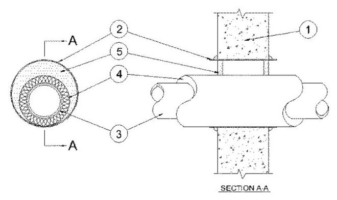
1. **Wall Assembly** — Min 6 in. thick reinforced lightweight or normal weight (100-150 pcf) concrete. Wall may also be constructed of any UL Classified **Concrete Blocks**\*. Max diam of opening is 14 in.
