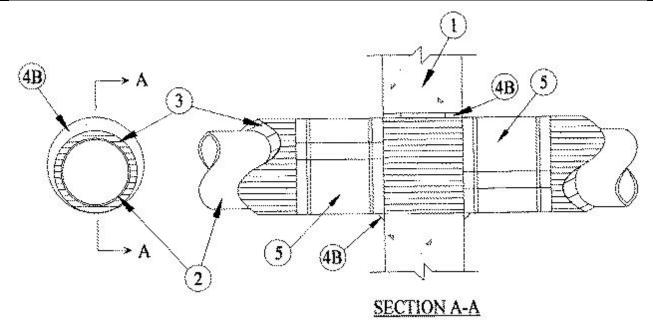
1. **Wall Assembly** — Min 6 in. (152 mm) thick reinforced lightweight or normal weight (100-150 pcf or 1600-2400 kg/m³) concrete. Wall may also be constructed of any UL Classified **Concrete Blocks\***. Max diam of opening is 18 in. (457 mm).
