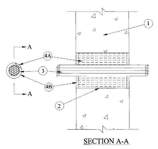
1. **Wall Assembly** — Min 6 in. thick reinforced lightweight or normal weight (100-150 pcf) concrete. Wall may also be constructed of any UL Classified **Concrete Blocks**\*. Max diam of opening is 4 in.
