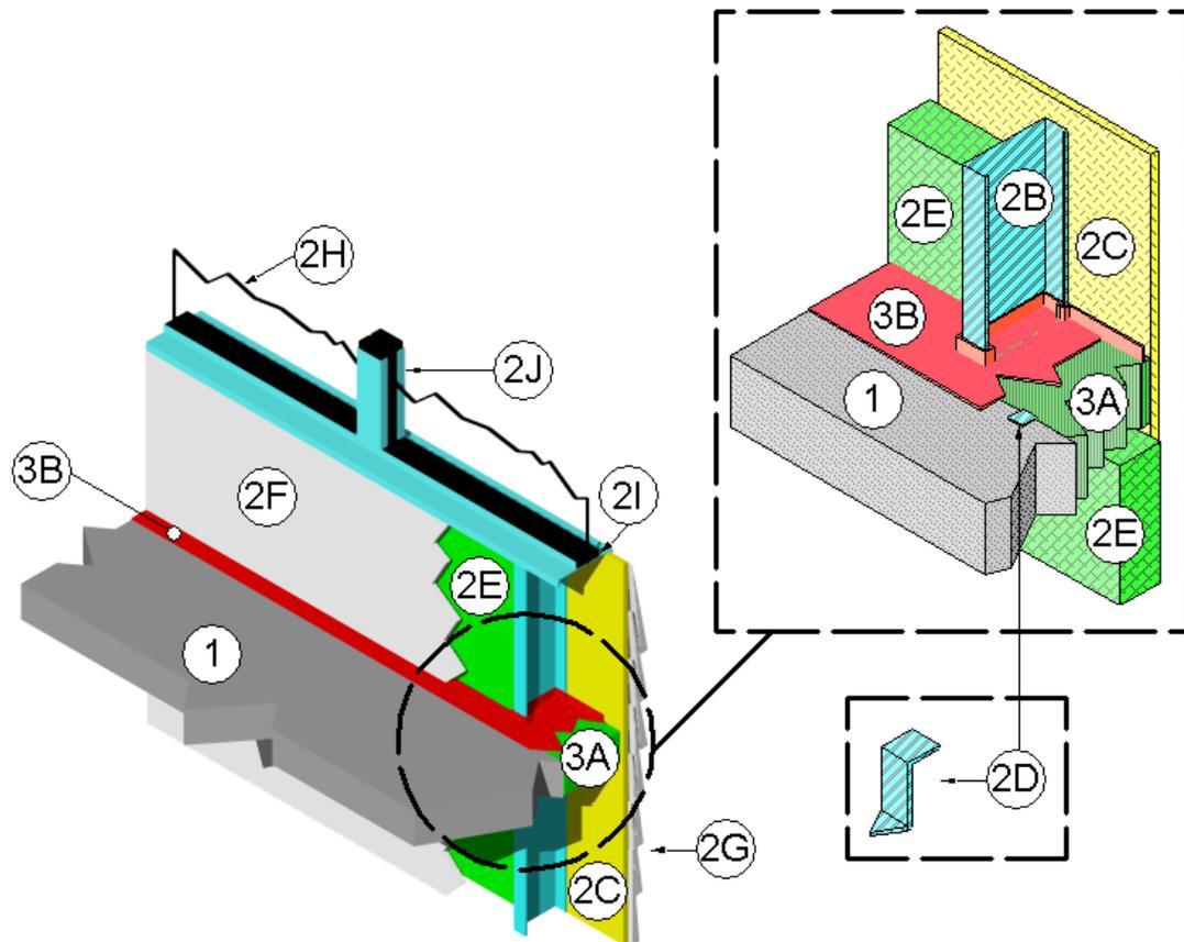
1. CONCRETE FLOOR ASSEMBLY: Two-hour rated concrete floor assembly made from either lightweight or normal weight concrete with a density of 100 to 150 pcf, having a min. thickness of 4-1/2 in. at the joint face. When a longitudinal recess (blockout) is required to contain an architectural joint system, increase
