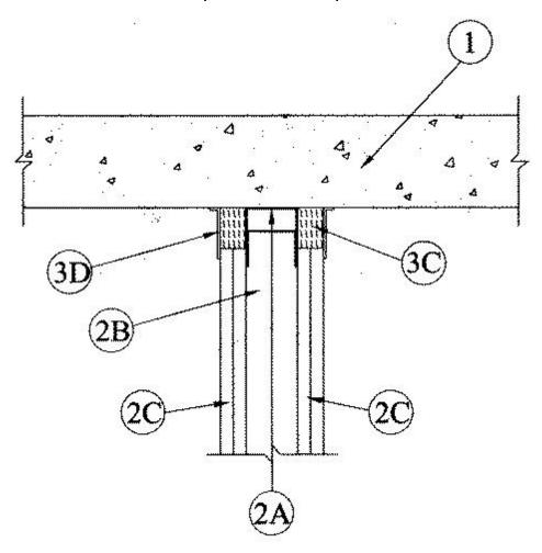
1. **Floor Assembly** — Min 4-1/2 in. thick steel reinforced lightweight or normal weight (100-150 pcf) structural concrete. Floor may also be constructed of any min 6 in. thick UL Classified hollow-core **Precast Concrete Units\***.
