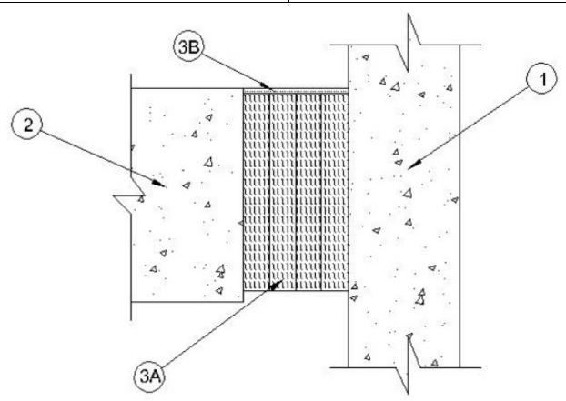
1. **Wall Assembly** — Min 4-1/2 in. (114 mm) thick steel-reinforced lightweight or normal weight (100-150 pcf or 1600-2400 kg/m³) structural concrete. Wall may also be constructed of any UL Classified **Concrete Blocks**\*.
