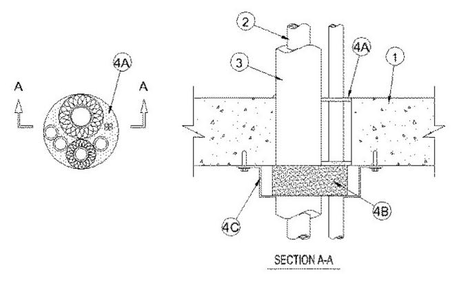
1. **Floor or Wall Assembly** — Min 4-1/2 in. (114 mm) thick reinforced lightweight or normal weight (100-150 pcf or 1600-2400 kg/m³) concrete. Wall may also be constructed of any UL Classified **Concrete Blocks**\*. Max diam of opening 6 in. (152 mm).
