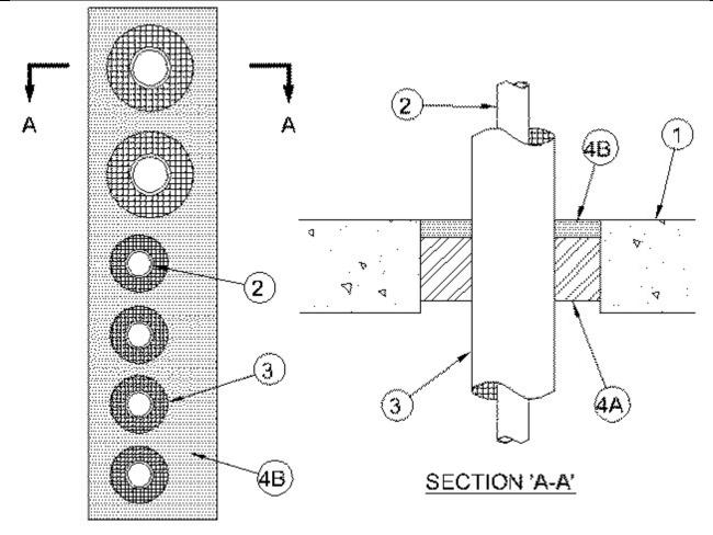
1. **Floor or Wall Assembly** — Min 4-1/2 in. (114 mm) thick reinforced lightweight or normal weight (100-150 pcf or 1600-2400 kg/m³) concrete floor or min 5-1/2 in. (140 mm) thick reinforced lightweight or normal weight concrete wall. Wall may also be constructed of any UL Classified **Concrete Blocks**\*. Max area of opening is 144 sq in. (929 cm²) with max dimension of 24 in. (610 mm).
