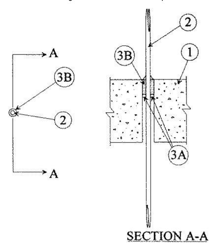
1. **Floor or Wall Assembly** — Min 4-1/2 in. thick reinforced lightweight or normal weight (100-150 pcf) concrete. Wall may also be constructed of any UL Classified **Concrete Blocks\***. Max diam of opening is 1/2 in.
