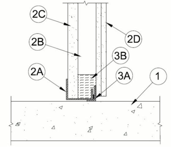
1. Floor Assembly — Min 4-1/2 in. (114 mm) thick reinforced lightweight or normal weight (100-150 pcf or 1600-2400 kg/m3) structural concrete. Floor may also be constructed of any min 6 in. (152 mm) thick UL Certified hollow-core Precast Concrete Units\*.
